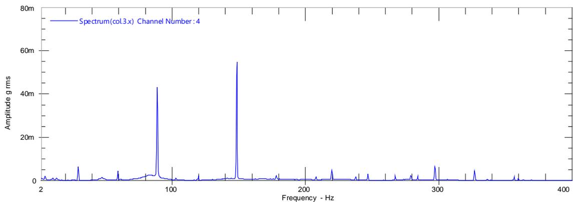
*Figure 10 Steady State Spectrum, Motor Lower Bearings*
