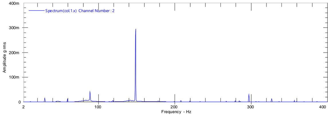
*Figure 9 Steady State Spectrum, Top of Pony Motor*
