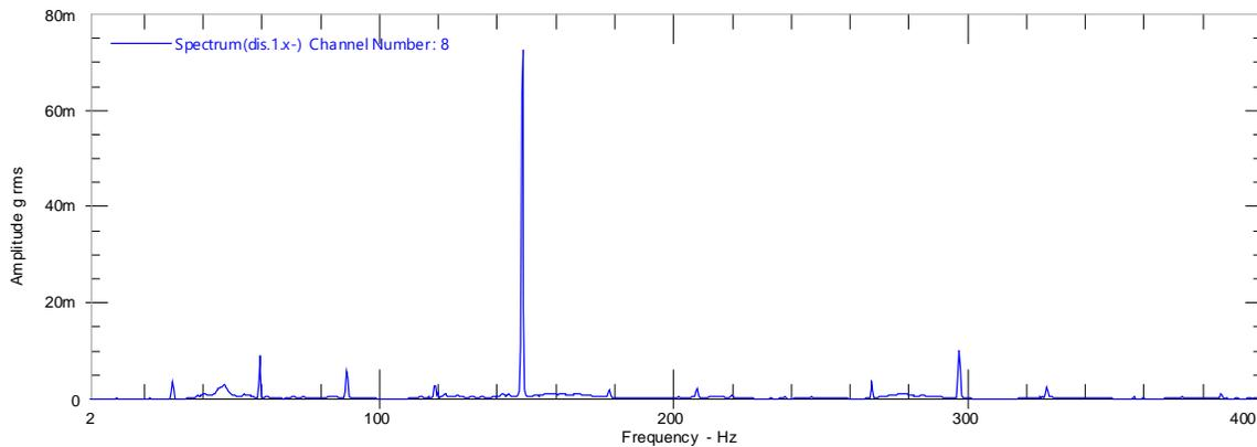
Figure 12 Steady State Spectrum, Discharge Piping
