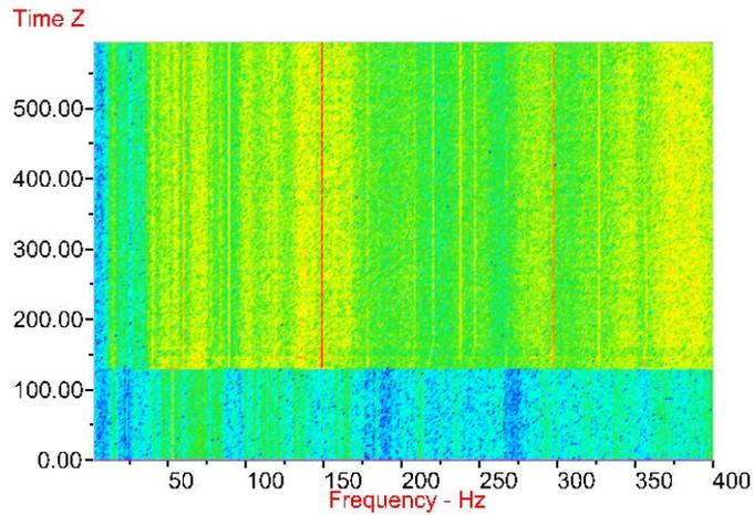
Figure 19 Transient, Suction Piping
