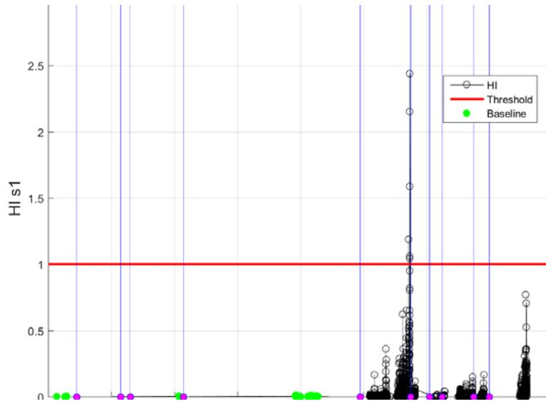
Figure 6. Health indicator result for one of the pumps in the field.
