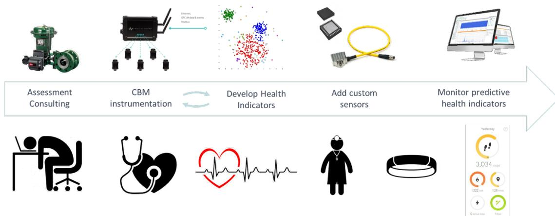
Figure 2 A process for development of CBM instrumentation on new equipment may start with analysis of existing data. A short-term pilot study should help determine whether new instrumentation (sensors) are needed or not.
