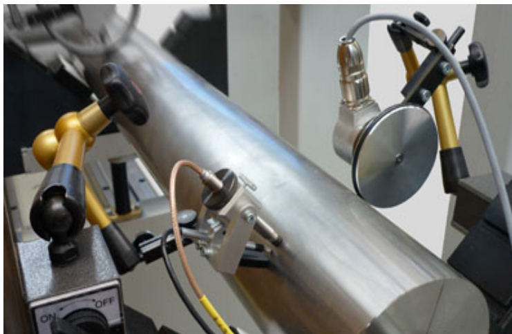
Fig 4 - Set up for Measuring electrical run out- courtesy Hoffmann
