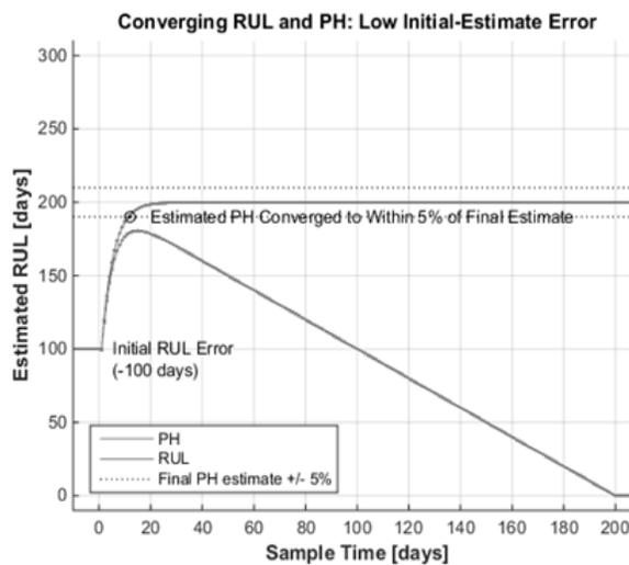
Figure 8: RUL and PH estimates when initial RUL is lower than actual
