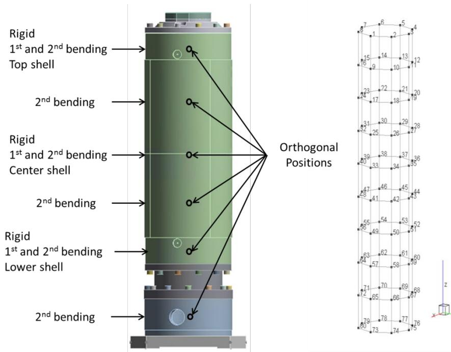
**Figure 3: : Suggested accelerometer locations (left) and actual location for the roving hammer empirical modal tests (right)**
