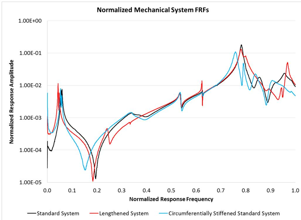
**Figure 5: Normalized FRFs of the standard system and modified system**
