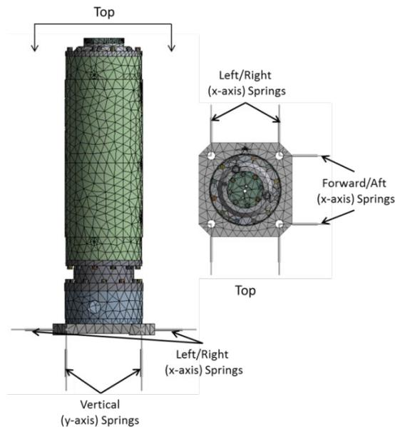
**Figure 2: Model mesh and spring to ground boundary conditions**
