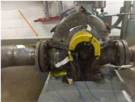
Figure 8: Suction Flange Accelerometer
