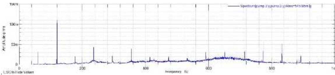
Figure 14: Steady State Outboard Pump Spectrum (Horizontal Radial)
