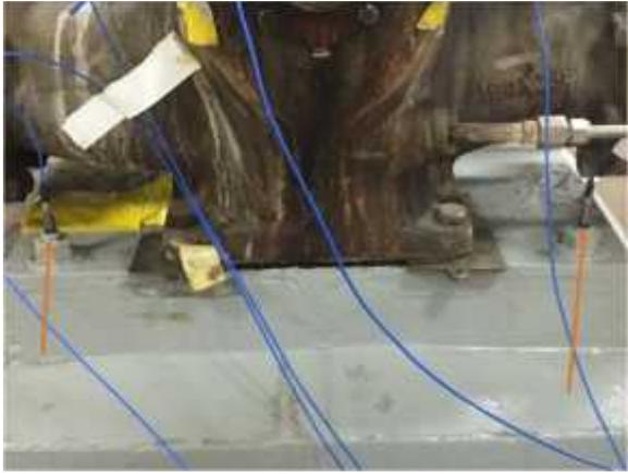
Figure 6: Base Bolt Accelerometers
