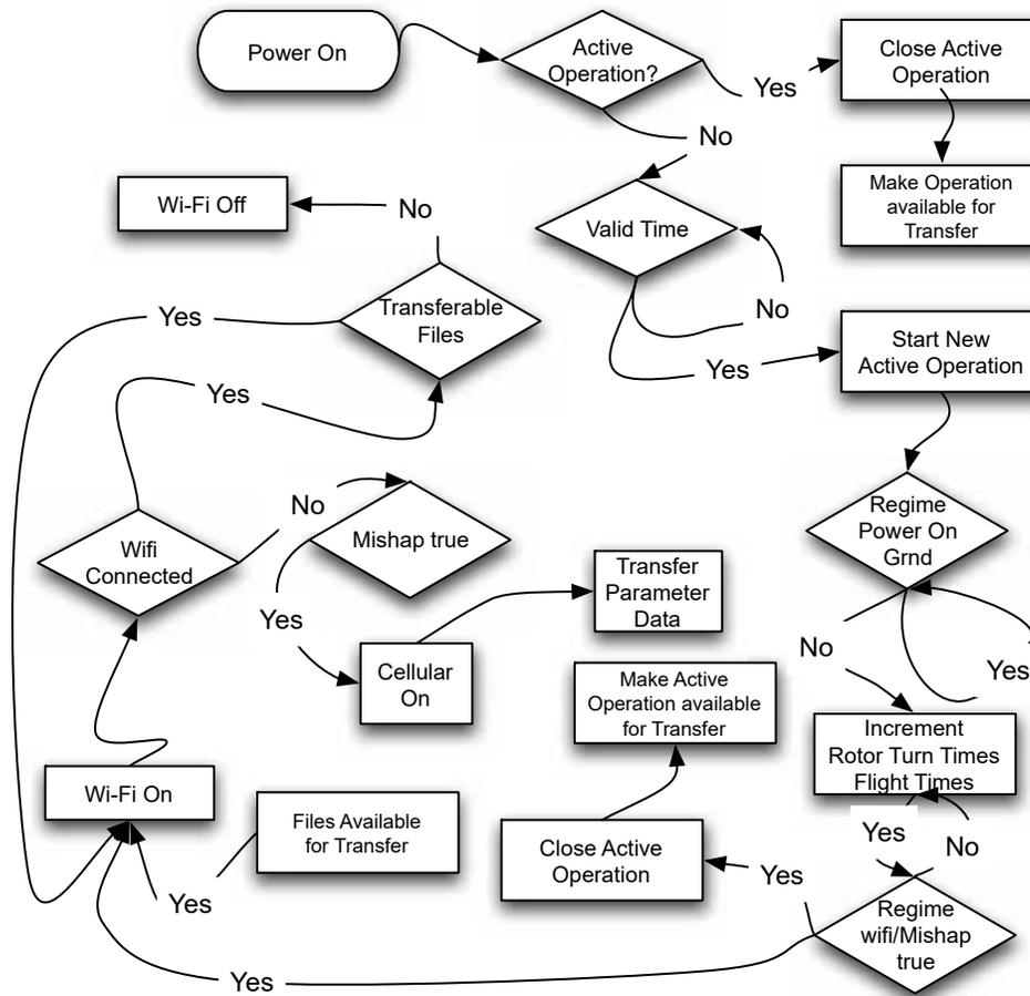
Figure 1 Operation Finite State Machine
