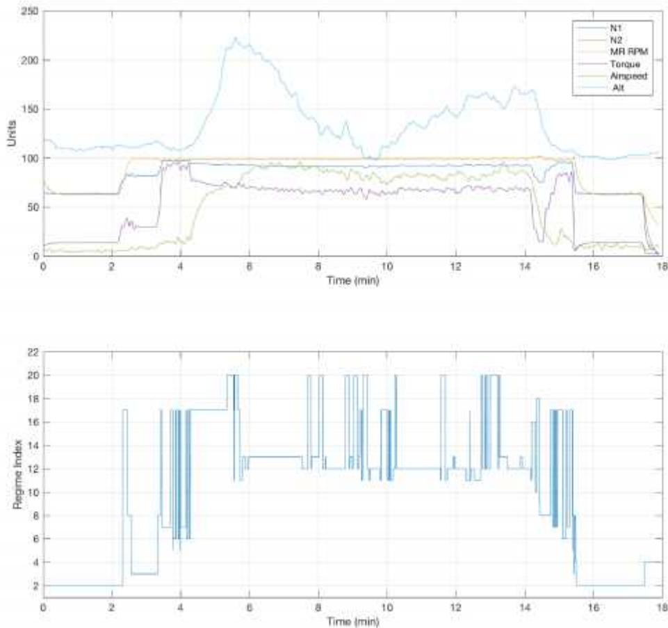
**Figure 3 Flight Parameters and Regime Index**
