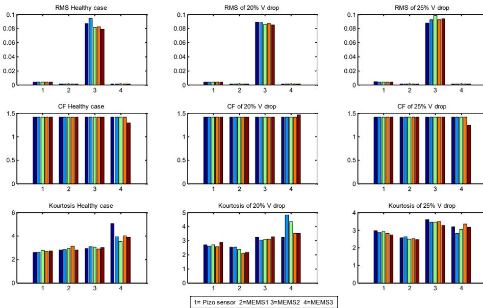
Figure 11 Time domain parameters: the motor at full load is equipped with various conditions (healthy, 20% & 25% V drop at 1500 rpm speed)
