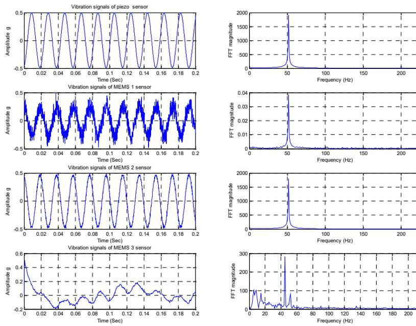
Figure 9 Measured acceleration responses by the MEMS accelerometers and the piezoelectric accelerometer at 55Hz for the excitation amplitude 0.7g
