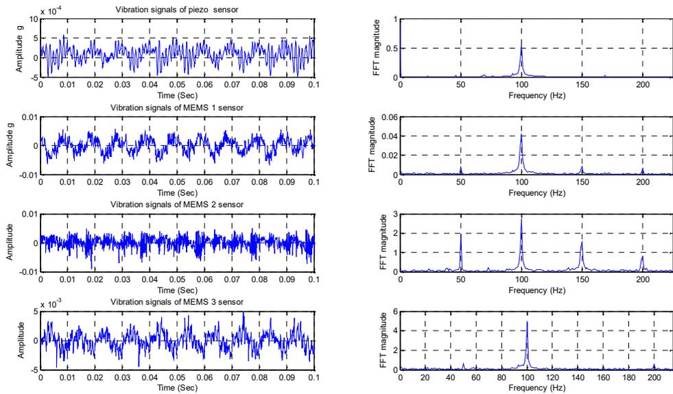
Figure 15 Time and Power spectra of the signal of the piezoelectric accelerometer and MEMS accelerometers. The motor at full load is equipped with 25% voltage drop at 1500 rpm speed.
