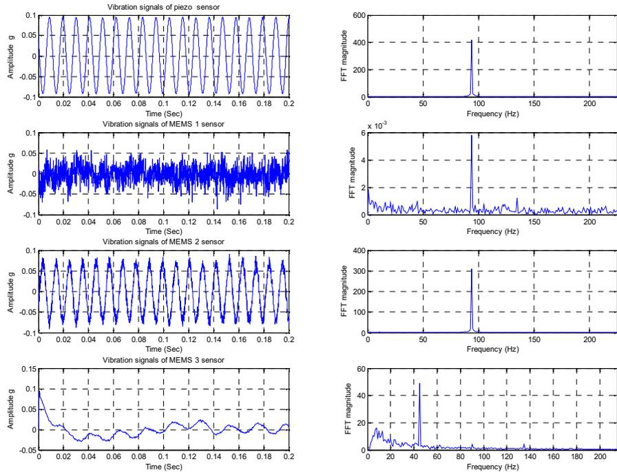
Figure 8 Measured acceleration responses by the MEMS accelerometers and the piezoelectric accelerometer at 95Hz for the excitation amplitude 0.2g
