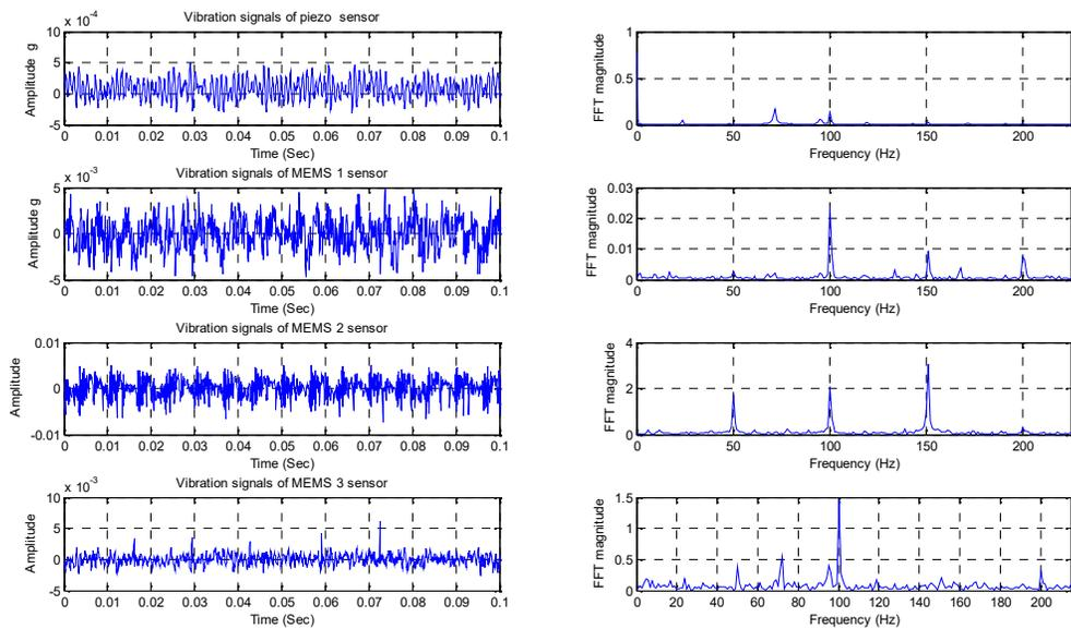
Figure 18 Time and Power spectra of the signal of the piezoelectric accelerometer and MEMS accelerometers. The motor at full load is equipped with 2mm misalignment at 1500 rpm speed.
