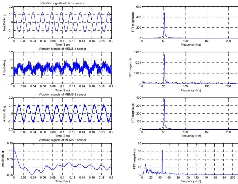
Figure 7 Measured acceleration responses by the MEMS accelerometers and the piezoelectric accelerometer at 55Hz for the excitation amplitude 0.2g
