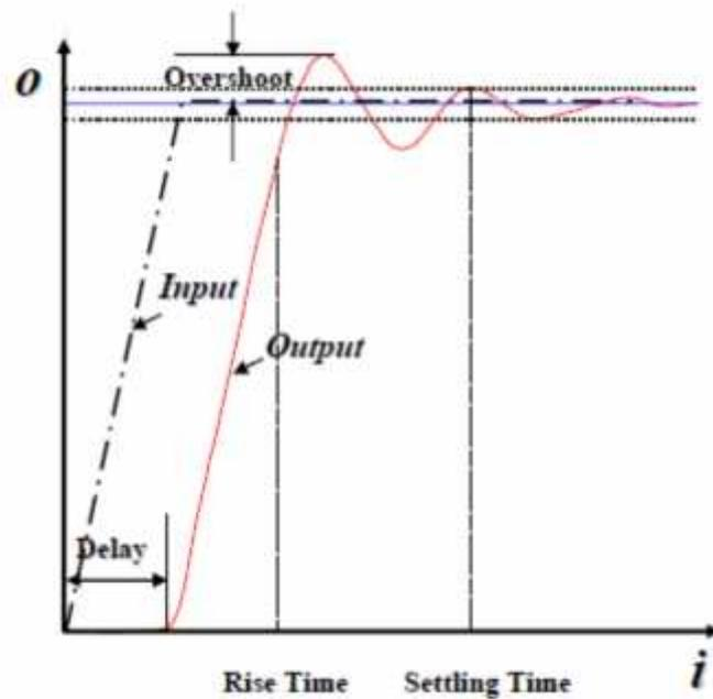
Figure 3 dynamic characteristics of sensor
