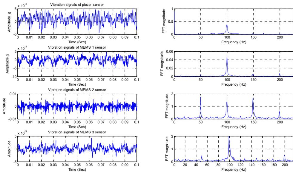
Figure 14 Time and Power spectra of the signal of the piezoelectric accelerometer and MEMS accelerometers. The motor at full load is equipped with 20% voltage drop at 1500 rpm speed.
