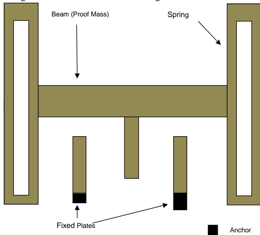
Figure 2 Capacitive MEMS accelerometer
