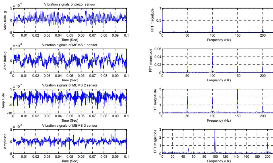
Figure 17 Time and Power spectra of the signal of the piezoelectric accelerometer and MEMS accelerometers. The motor at full load is equipped with 1mm misalignment at 1500 rpm speed.
