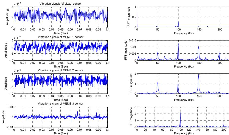
Figure 13 Time and Power spectra of the signal of the piezoelectric accelerometer and MEMS accelerometer. The motor is at full load and 1500 rpm speed
