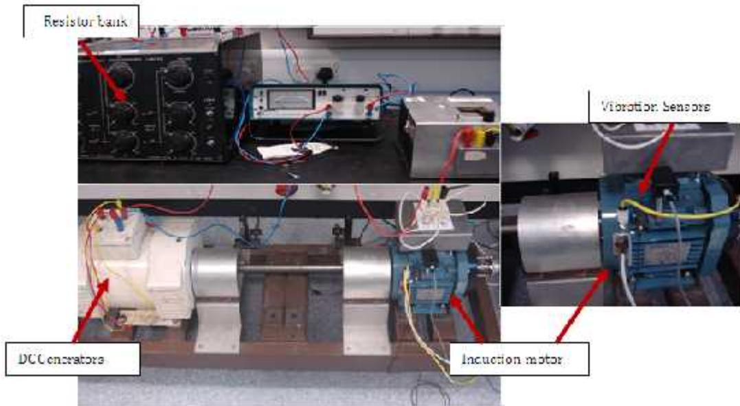
Figure 4 Schematic diagram of induction motor test rig
