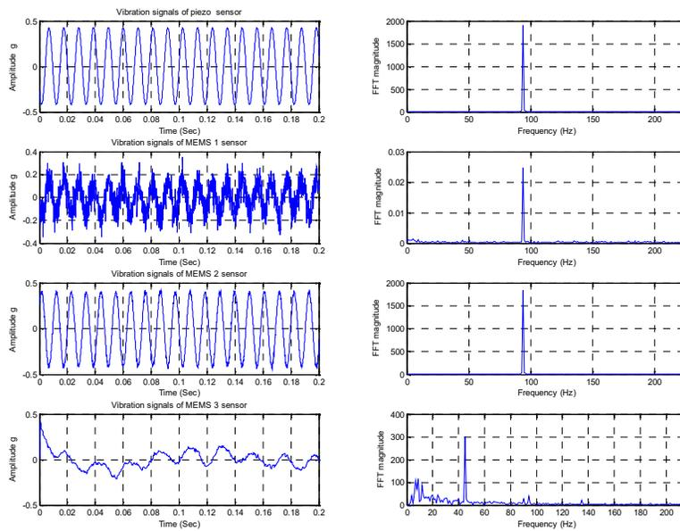
Figure 10 Measured acceleration responses by the MEMS accelerometers and the piezoelectric accelerometer at 95Hz for the excitation amplitude 0.7g
