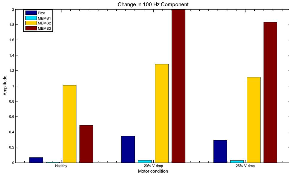
Figure 16 Changes in 100Hz components from healthy and 20% & 25% voltage drop. The motor is at full load and 1500 rpm speed.
