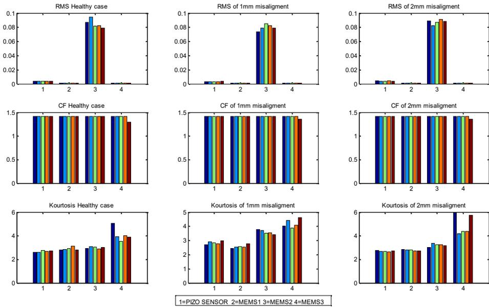
Figure 12 Time domain parameters. The motor at full load is equipped with various conditions (healthy, 1mm & 2mm misalignment at 1500 rpm speed)
