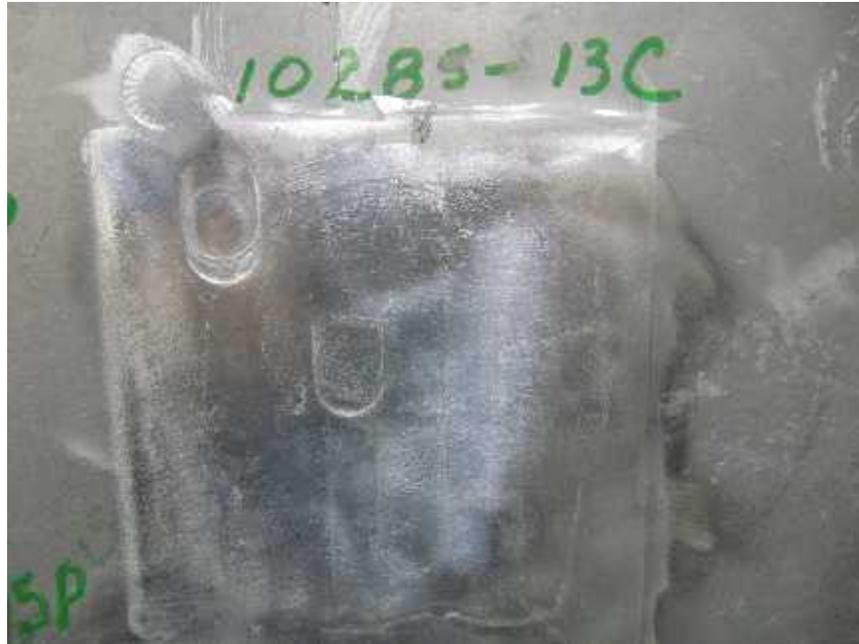
Figure 8 Typical filled hole ground smooth with a fly cutter tool, followed by a ½-inch end mill, and surface sanded using an air Dymet® sander and Scotch Brite® pads.
