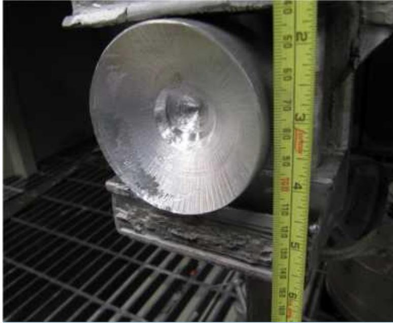
**Figure 1** Test coupon utilized to determine feasibility of cold spray repair of the armor plate.
