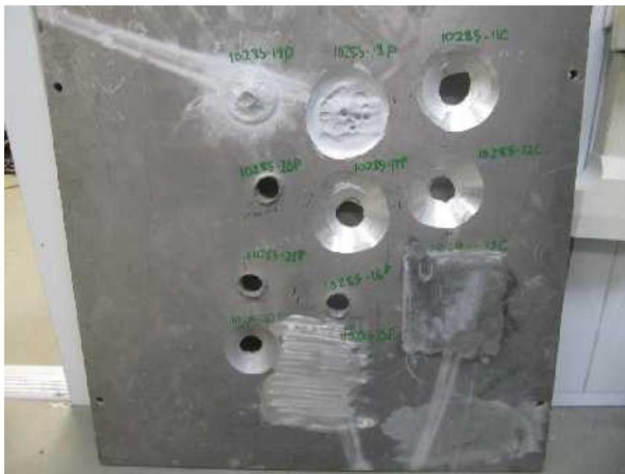
Figure 9 Similar to Figure 10, a filled hole ground smooth with a fly cutter tool, followed by a ½-inch end mill and surface sanded using an air Dymet® sander and Scotch Brite® pads.
