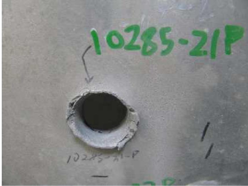
**Figure 4** Typical ballistic damage noted on the as-received aluminum armor plate.
