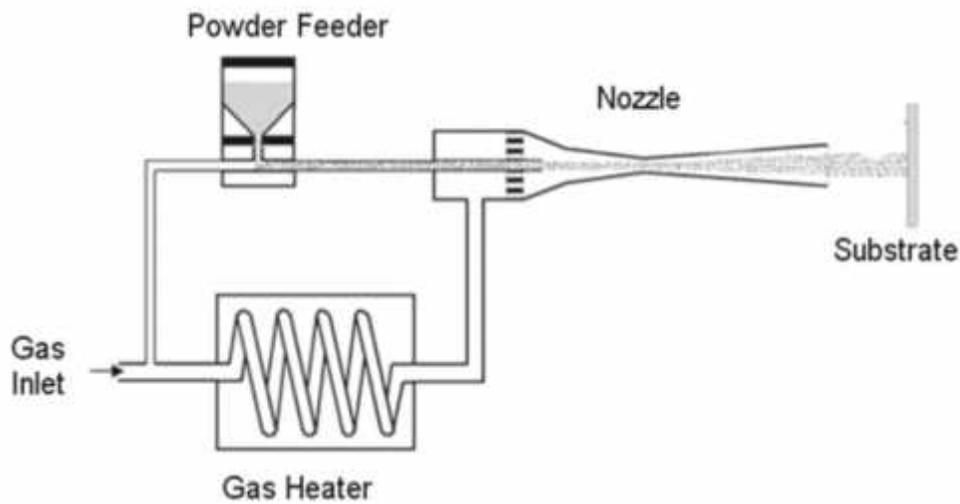
**Figure 1 Schematic of a typical cold-spray assembly**
