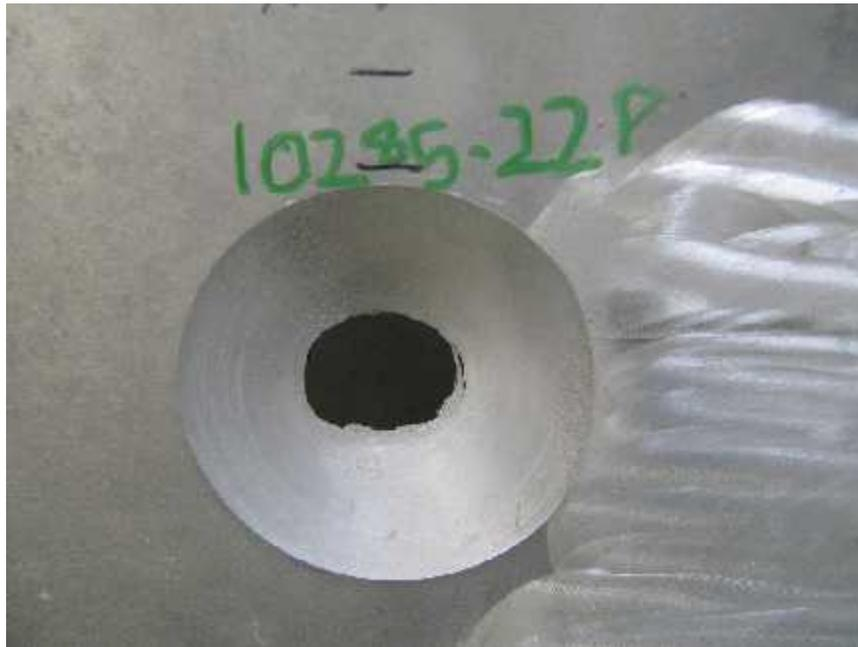
**Figure 5** Chamfering of hole to allow for better cold spray adherence.
