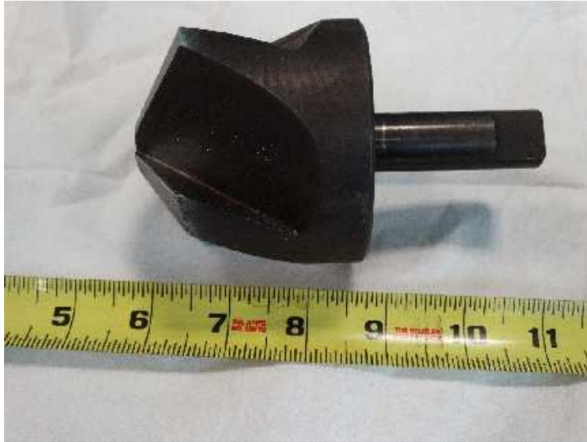
**Figure 6** Tool utilized to chamfer projectile holes in preparation of cold spray fill.
