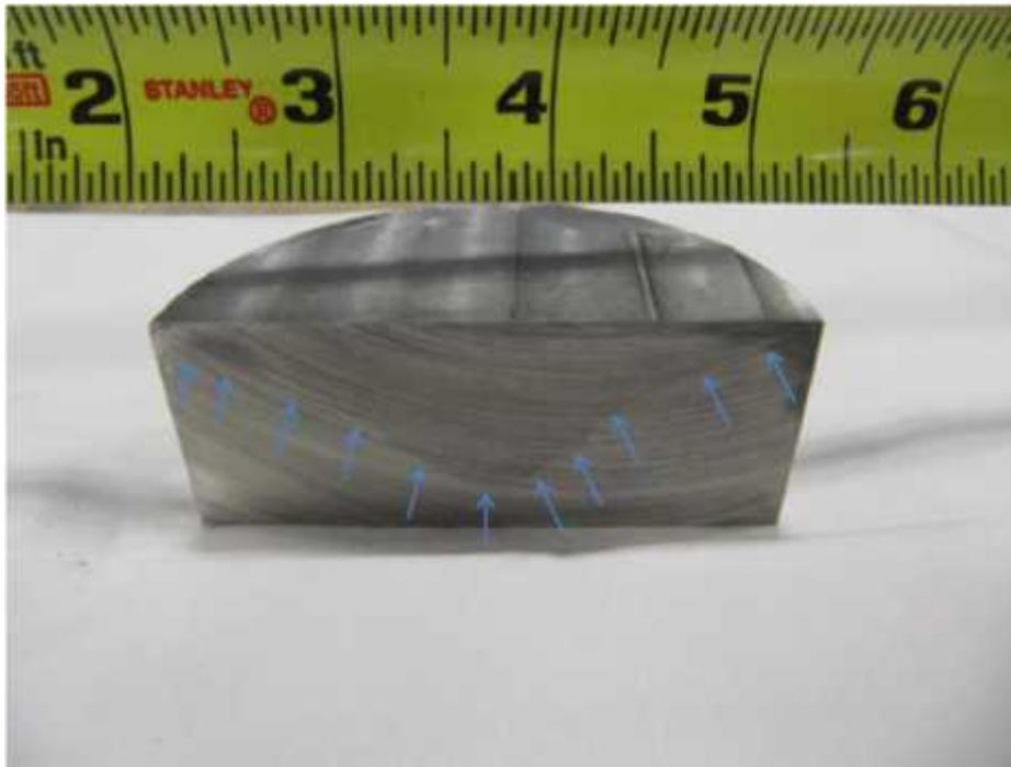
**Figure 2** Cross section of test coupon showing cold spray fill (region above arrows).
