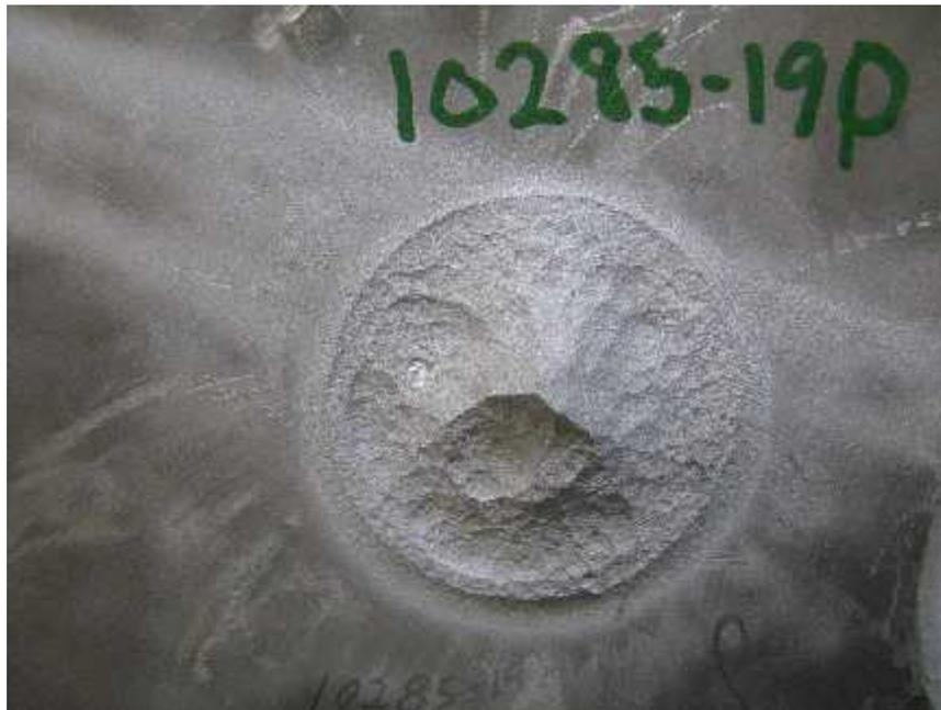
**Figure 7** Typical hole filled with cold sprayed aluminum powder.
