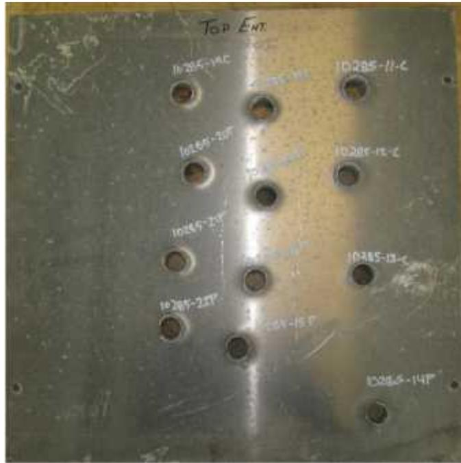
**Figure 2 As-received damaged AA5083 plate prior to cold spray repairs.**
