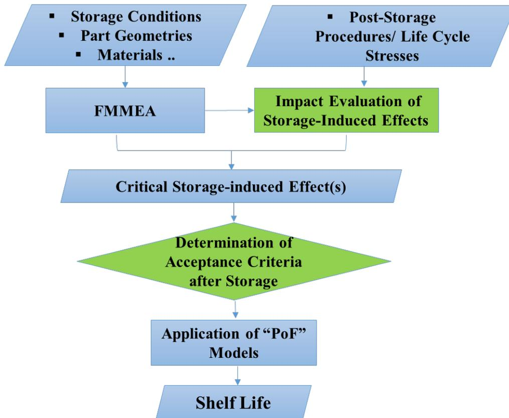
Figure 1. Physics of Failure Shelf Life Estimation Approach
