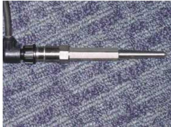
Figure 5. Stainless steel probe (stinger)
