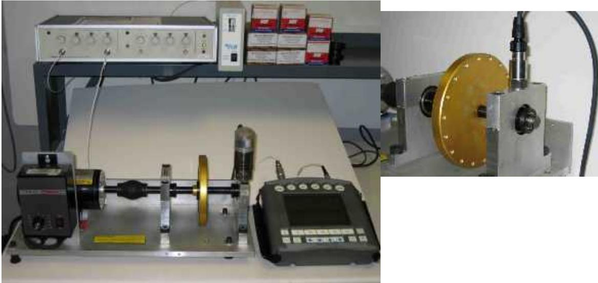
Figure 17: Rotor kit test setup with inlay photo of the 622B01 accelerometer
